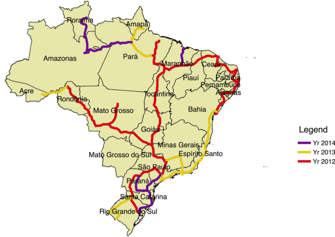
Figure 2: New broadband backbones implemented as part of PNBL: 2012-2014
